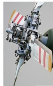
**The tail rotor rotates at high speed.**
