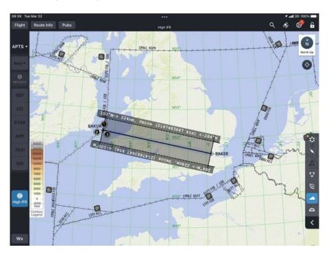
Manual Waypoint entry to the FMS requires the highest flight crew coordination and discipline to prevent navigational errors. Pilots should consider requesting a phonetic spelling of a Waypoint from ATC, that is not already loaded in the FMS.
