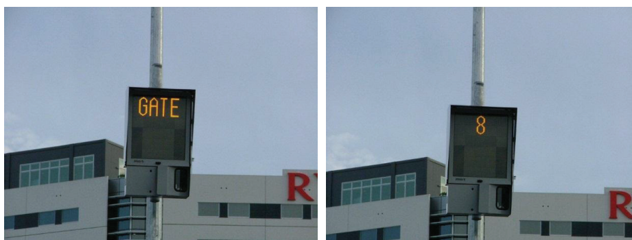
Alternating display of Gate Number in Standby mode.
