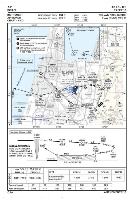
On the incidents investigated, it was revealed that the crews did not notice there was more than one option to choose from for an arrival to RWY 26 via KEREN, and the incorrect approach was selected in the FMS. As a result, the aircraft flew an incorrect path both laterally and vertically. The terminology of the ATC for the Visual Approach (with prescribed track) is "KEREN Approach", which might have contributed to the confusion of the crews.
